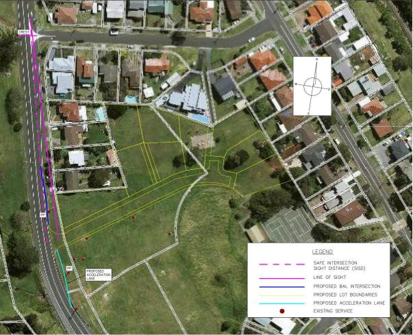
Figure A1: Required Safe Sight Distance (SISD) for proposed intersection
