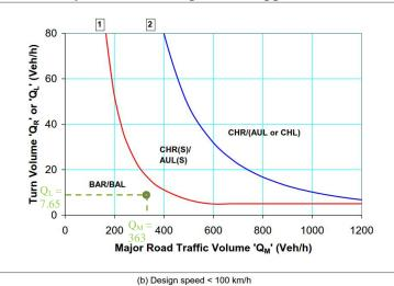
Figure 1: Determination of Intersection Treatment (Adapted from Guide to Road Design Part 4A – Unsignalised and Signalised Intersections)
